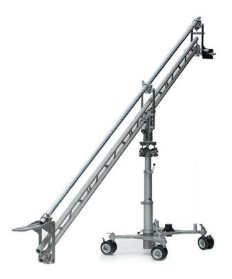
OctoJib is a basic, **lightweight & modular jib**, able to support light camera or Gimbal packages. The main parts are composed with octogrip bilite, pipe and couplers, already used by grip crew for several years as tracks beams, wall-spreader, rigging tools, sliders.
